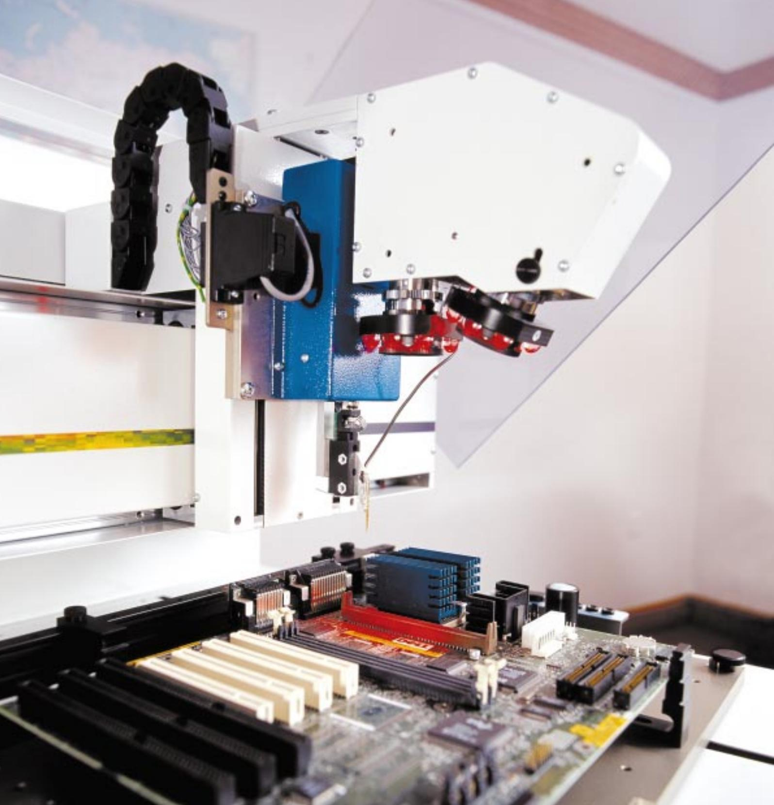
High value boards, legacy systems, new fine pitch SMD based assemblies present you with a seemingly endless series of repair challenges. The new GRS500 from Polar is designed especially to meet the challenges of service and repair departments faced with troubleshooting a wide variety of board technologies.
